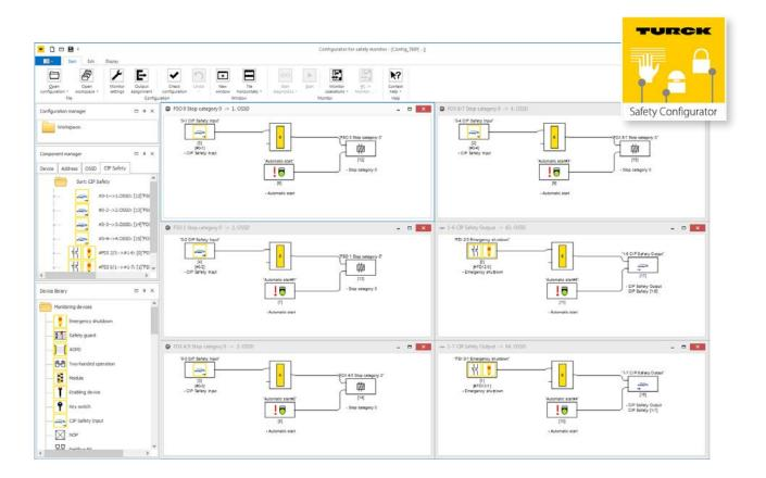
The Turck Safety Configurator also allows an online connection to a safety device to view the active diagnostic status of each safety signal and logical function during machine operation in real time.
